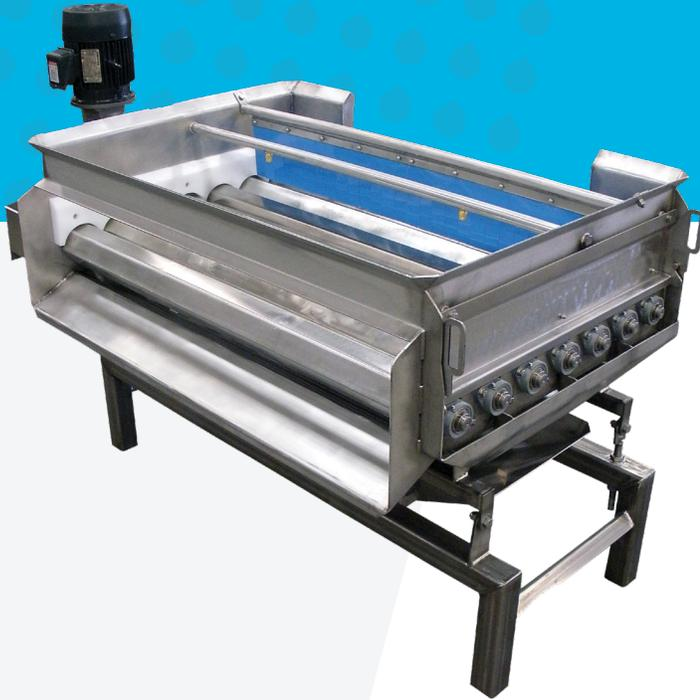
The Hex Spreader evenly spreads product across the full width of the discharge while removing undersized product, debris and excess water. Spreading into single layer gives you the best presentation of product for optical sorting and sizing. The top grill cover provides clear visibility and full wash through capability – improving sanitation and reducing downtime.
